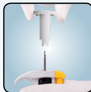
Insert the calibration key and locate in the key slots. The calibration key is delivered with the pipette.
